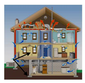
When a home is heated in the winter, warm air rises and leaks out of holes at the top of the home will cold air leaks in at the bottom to replace it.
