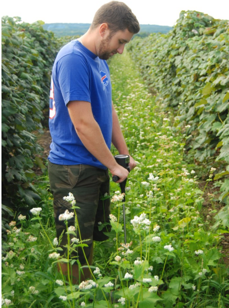
Scott Ebert measures soil compaction in a Concord vineyard with a cover crop planted in the row center. The cover crop mix consists of buckwheat, tillable radish, triticale, and crimson clover.
